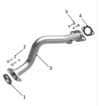
(Carefully read all instructions before installation) Disconnect the vehicle's battery before removal of the OEM exhaust system. This will prevent electrical accidents and will reset the computer if it applies to the vehicle. Remove existing front pipe from the vehicle. Only remove parts that will be replaced. Clean existing flange with a wire brush to ensure proper sealing.
